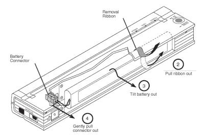
Figure 13. Instructions for removing the battery
